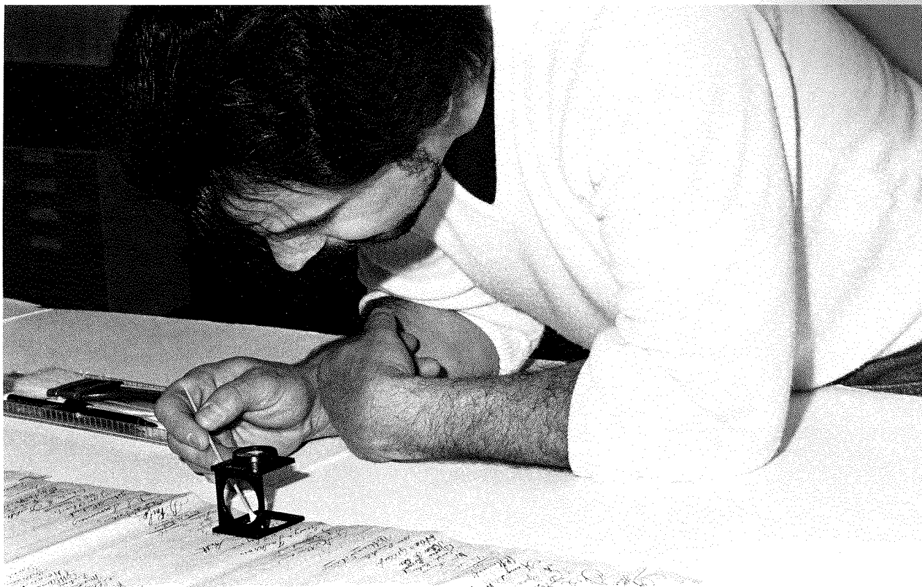
Blagoje Siljegovic, a conservator aide in the document conservation lab, tests the solubility of inks on an 1832 petition to the House of Representatives; the petition requests protection for the treaty rights of Cherokee Indians. Cleaning, repairing, and flattening a document of this size (128 feet) can take as long as 3 weeks. (Photograph by Nancy Olds.)
